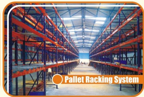
Pallet Racking System
